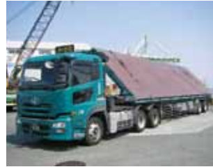
Land transportation of steel plate
